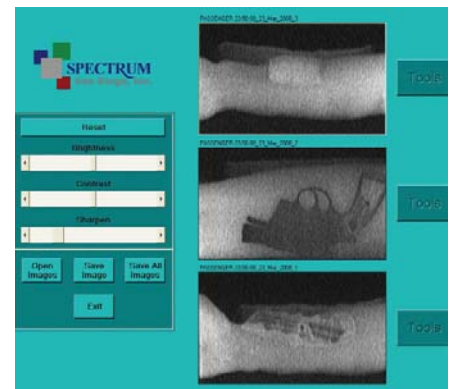
CastScope's system uses X-ray backscatter technology to scan medical casts, bandages and prosthetic limbs
