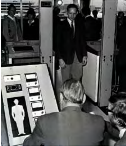
35 years on and the archway metal detector is still the primary method of screening passengers
